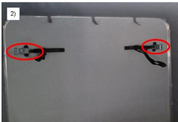
3. Then, pull down the roof shell of the vehicle slowly (view onto the rear end).
