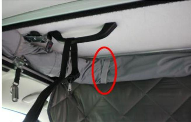
7. Close the Velcro® fastener of the access cover above the cabin.
