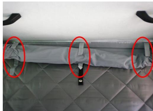
3. Open Click-Lock of the sleeping roof (driver's side as well as passenger's side)
