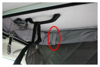
7. Close the Velcro® fastener of the access cover above the cabin.
