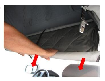
2. Fold up the recumbency device downwards before closing the roof (picture 1).
