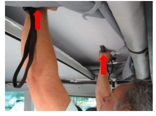
6. If needed, the access cover can be reeled in and fixed with the marked push button.
