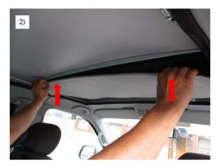
8. Finally, parts, which are projecting laterally, can be accommodated in the cavity between sleeping roof and access cover.
