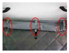
3. Open Click-Lock of the sleeping roof (driver's side as well as passenger's side)
