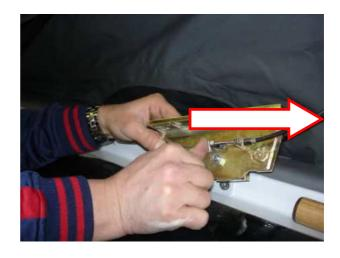
If the lock does not run clearly across the plugs, you will have to readjust it. For doing so please unfasten both locknuts.
