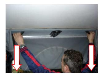
5. Pullonce more strongly to the bottom with both hands at the left and right handle respectively until the roof shell engages fort he second time.
