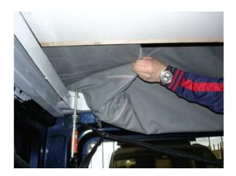
4. Pull constantly to the bottom with both handles until the roof shell engages audibly once.
