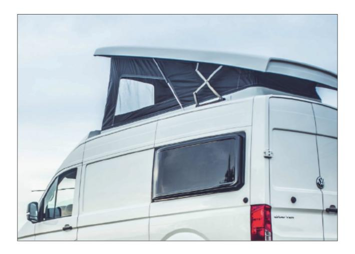
Supplied in gel coat white - the recommendation is to paint the product before use to protect the fibreglass and avoid age and discolouration.
